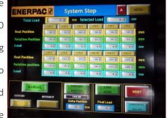
operation the operator can check the load and the stroke of each cylinder. The Cylinder Accuracy is ± 3%. Jacking Layer under Climbing Jack Frame (CJF) made by steel blocks is easily handled by operator / riggers (with a maximum weight of 20 kg for each steel).
